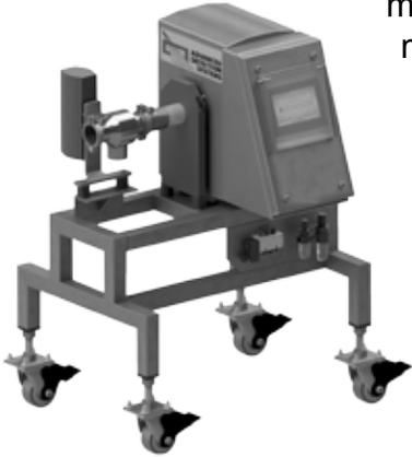
Pipeline applications involve the installation of a non-metallic pipe section that sends product through a metal detector for testing. Pipeline applications are used where the extra sensitivity of a small aperture outweighs the benefit of final package inspection. An example would be testing soup before it reaches a packaging line using metal cans.
