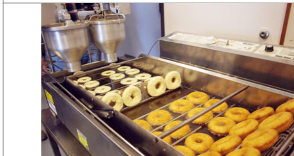
Mark VI Deep with Dual Automatic depositors (for Ring donuts only)
